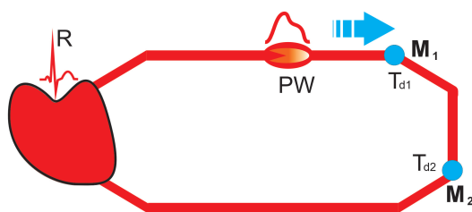
Fig. 1. Principle of BP measurement by the PTT method
