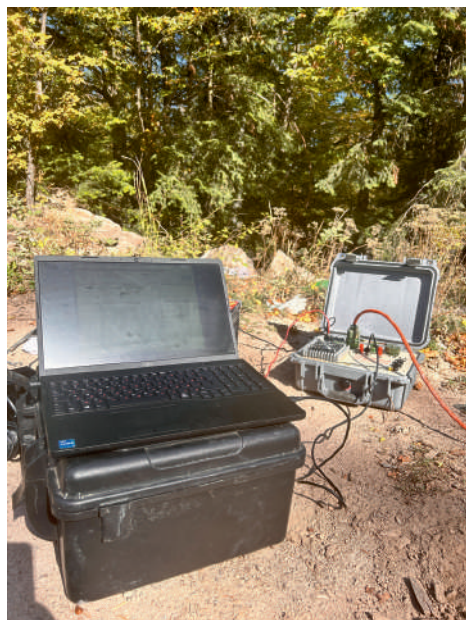
Fig. 2. Field survey view – equipment ZZ Universal 96-Channel Resistivity/IP Meter
