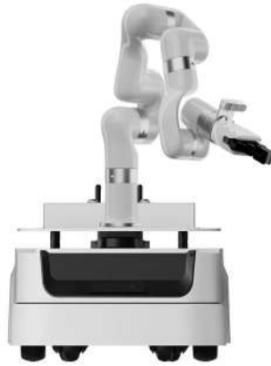
Fig. 2. Robot Athena 2 with robotic arm and gripper
