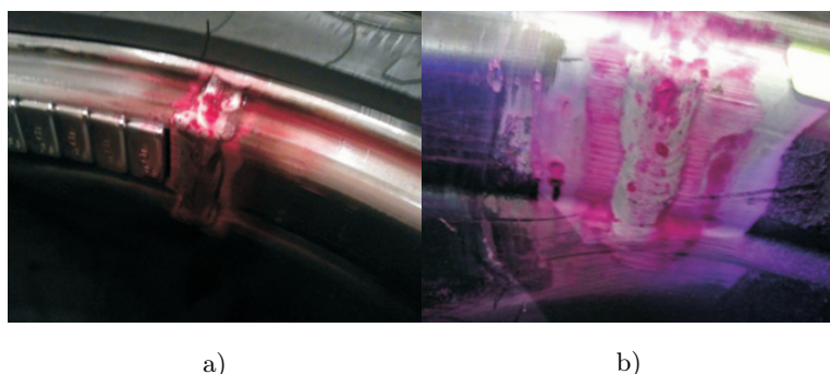
Fig. 1. PT control of welding joints a), and b) \times 5
