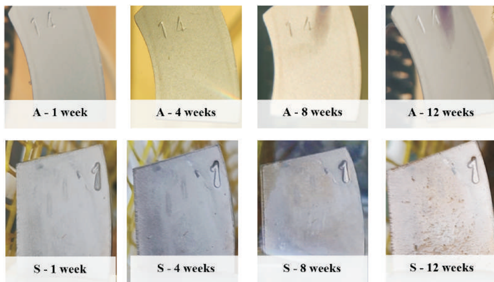
Fig. 4. Ni+2%Ag coating after a stay in a simulated marine environment – aquarium (A); in a natural marine environment (S)
