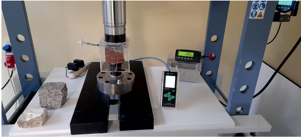
Fig. 1. System for investigating the emissions of fine dispersed mineral particles under uniaxial deformation of rock specimens
