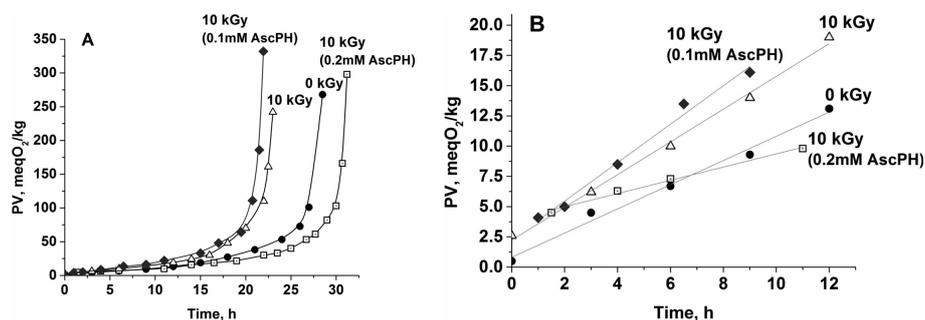
Fig. 2. Kinetic curves of LOOH accumulation during autoxidation of oil extracted from gamma-irradiated peanuts before and after addition of 0.1 mM and 0.2 mM ascorbyl palmitate (AscPH) for (A) the whole oxidation process and (B) for the initial stage of oxidation
