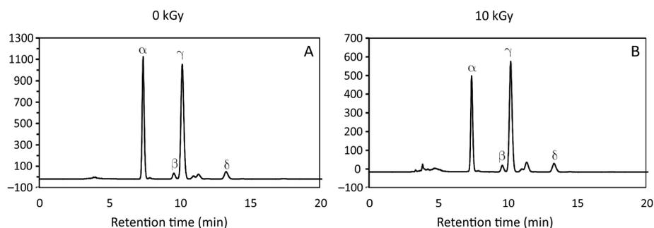
Fig. 1. HPLC chromatograms of  $\alpha$ -,  $\beta$ -,  $\gamma$ - and  $\delta$ -tocopherols in peanut oil obtained from (A) non-irradiated (0 kGy) and (B) irradiated (10 kGy) peanuts
